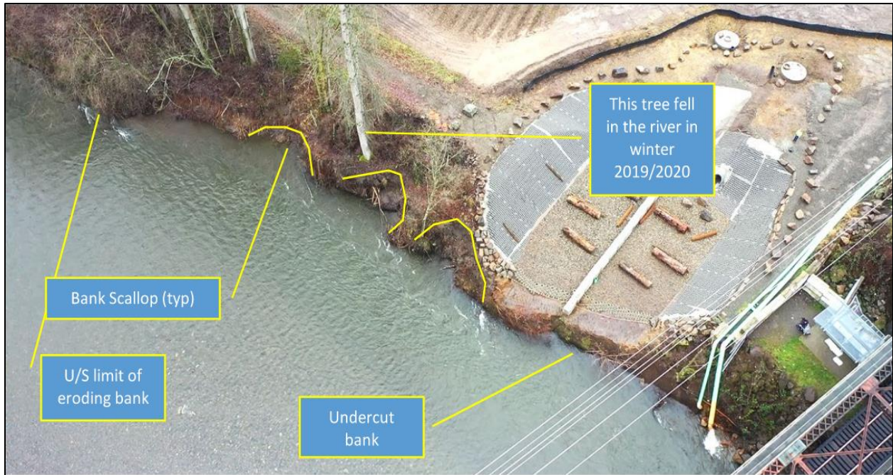
Figure 4-20. December 2019 UAV image annotated with erosional features. The riverbank shown above waterward of the edge of outfall has slumped or eroded back 5-10 feet since this photo was taken.
